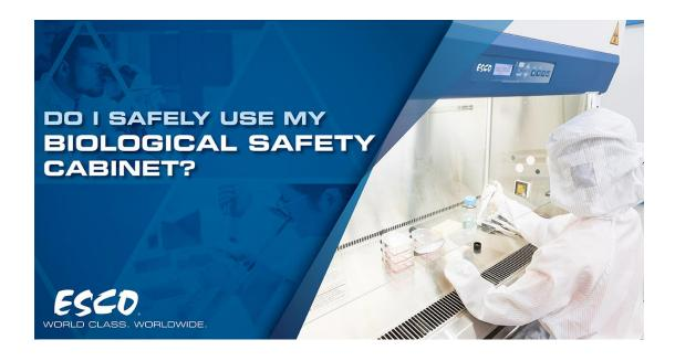
Biological Safety Cabinet is a primary engineering control which provides user protection against biohazards as the inflow air creates airflow barrier preventing accidental release of biohazards from the cabinet's working area and at the same time provides product protection with the airflow barrier inside the work zone created by the downflow air. Hand in hand with this are the proper laboratory practices for optimum safety.
